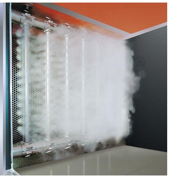
or ceiling. It is important to maintain a minimum distance from the floor of 85mm and 165mm from the ceiling. This is to avoid creating turbulence that could direct the steam onto the ductwork, resulting in condensation. The minimum duct height a steam lance can be used in is therefore 250mm.
